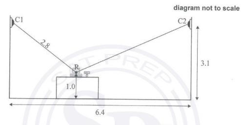
The cameras are positioned at a height of  $3.1 \,\mathrm{m}$ , and the horizontal distance between the cameras is  $6.4 \,\mathrm{m}$ . The cash register is sitting on a counter so that its centre, R, is  $1.0 \,\mathrm{m}$  above the floor.
